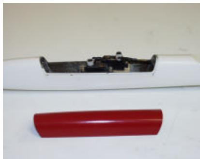
The shape of a part can be easily changed or a new part prototype created using Chevant Clay and Sheet Wax as pattern making materials. As an example of the process I will modify the shape of the hatch on an RC glider model.
