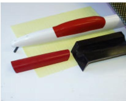
Let the completed mold cure overnight. Remove the Mylar sheets, original part and clay from the mold and trim the edges of the mold off with a Dremel tool and a reinforced cut off wheel.
