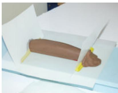
After the part is reshaped the mold making and molding of the part is the same methods used in our other tutorials. The bottom surface and ends of the mold are created with small sheets of .014" Mylar and a scrape foam block. The parts are held together with more clay and a few bits of bag sealant tape. Partal High Temp wax and Safelease 30 mold releases were used to prepare the surfaces before the mold is started.
