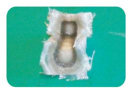
strength use a milled glass filler. Brush the mixture into the corners and let it cure to a solid that is only slightly tacky on the surface you will have to wait about 2 to 3 times the pot life of the epoxy. Then wet out the surface of the mold with another batch of epoxy and lay in the glass cloth. CST style 3733 glass cloth has a course weave that wets out easily and conforms to shapes well.
