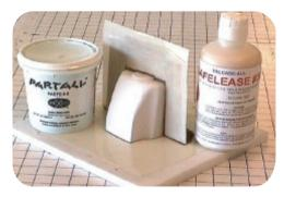
If you have any doubt about the surface, add a couple more layers of wax. The epoxy will lock into these imperfections if you don't use enough wax. Then apply a complete layer of liquid mold releases. I recommend the Safelease products as they can be wiped on with a cloth and dry in about 30 minutes.
