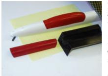
Let the completed mold cure overnight. Remove the Mylar sheets, original part and clay from the mold and trim the edges of the mold off with a Dremel tool and a reinforced cut off wheel.
