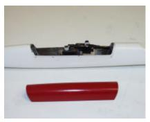
The shape of a part can be easily changed or a new part prototype created using Chevant Clay and Sheet Wax as pattern making materials. As an example of the process I will modify the shape of the hatch on an RC glider model.
