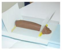
After the part is reshaped the mold making and molding of the part is the same methods used in our other tutorials. The bottom surface and ends of the mold are created with small sheets of .014" Mylar and a scrape foam block. The parts are held together with more clay and a few bits of bag sealant tape. Partal High Temp wax and Safelease 30 mold releases were used to prepare the surfaces before the mold is started.
